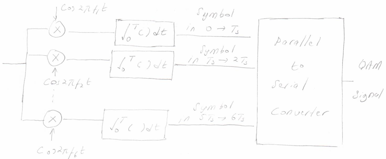
Note that which symbol is placed on which subcarrier depends on the stream of QAM signal
